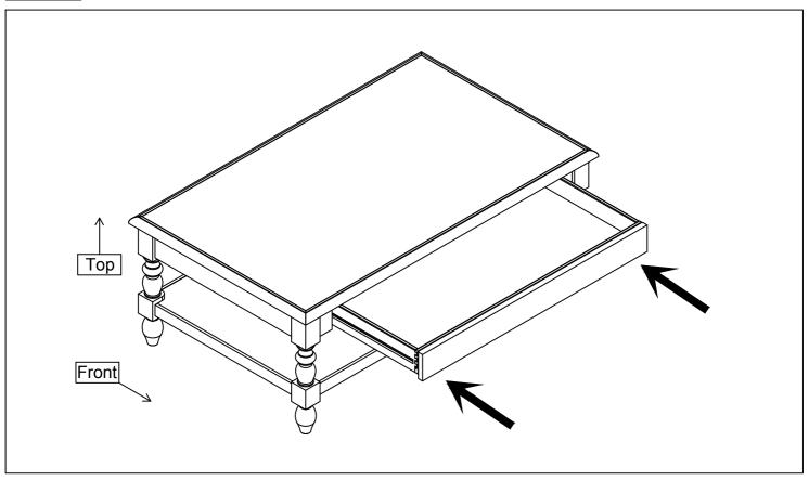
Turn the assembled unit upright. Re-install Drawer into Table Top (A).
