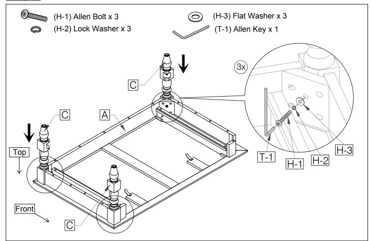
Position and secure 3 Legs (C) into corners using Allen Bolts (H-1), Lock Washers (H-2) and Flat Washers (H-3), stacking the hardware in the order as shown. Fully engage all bolts using Allen Key (T-1) but do not tighten them yet.
