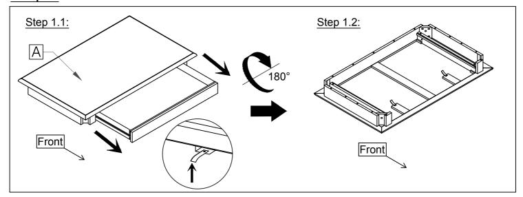
Step 1.1: Place Table Top (A) down onto a padded, non-marring surface. Pull drawer out and press upwards on the plastic drawer stop inside to completely remove drawer.
