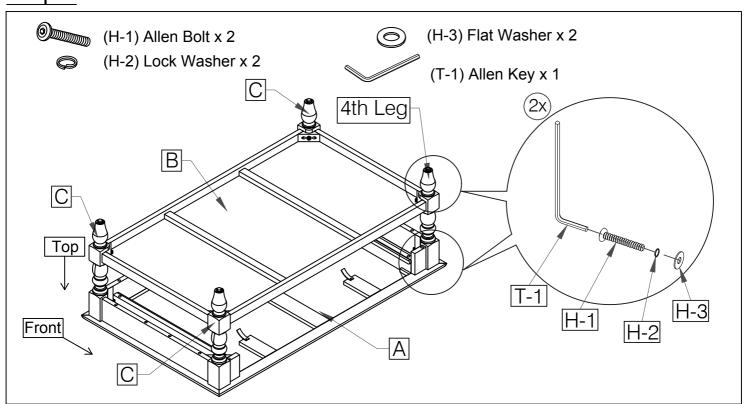
Install the leg 4th (C) into the assembled unit and secure with Table Top (A) and Shelf (B) using Allen Bolts (H-1), Lock Washers (H-2) and Flat Washers (H-3), stacking the hardware in the order as shown. Fully engage all bolts using Allen Key (T-1) but do not tighten them yet.
