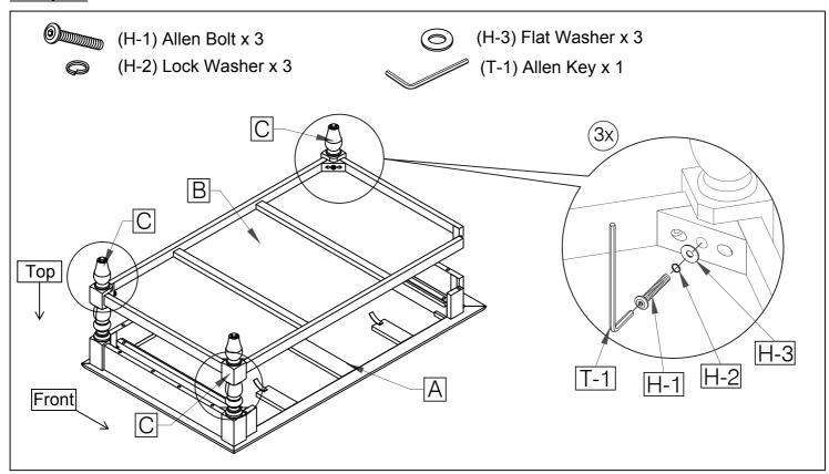
Position Shelf (B) into notches on each installed Legs (C) and secure using Allen Bolts (H-1), Lock Washers (H-2) and Flat Washers (H-3), stacking the hardware in the order as shown. Fully engage all bolts using Allen Key (T-1) but do not tighten them yet.
